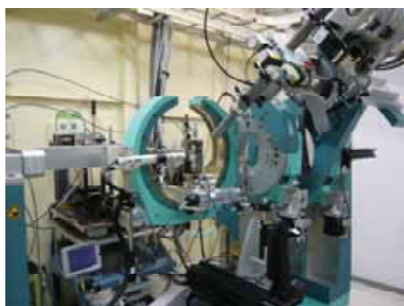
Fig.1 Multi-axial diffractometer on BL46XU
